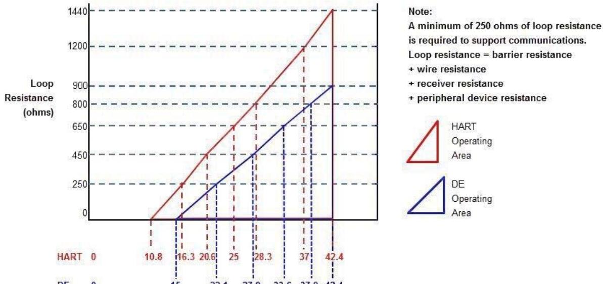
For DE,  $R_{max} = 35^* \text{ (Power Supply Voltage-15)}$
