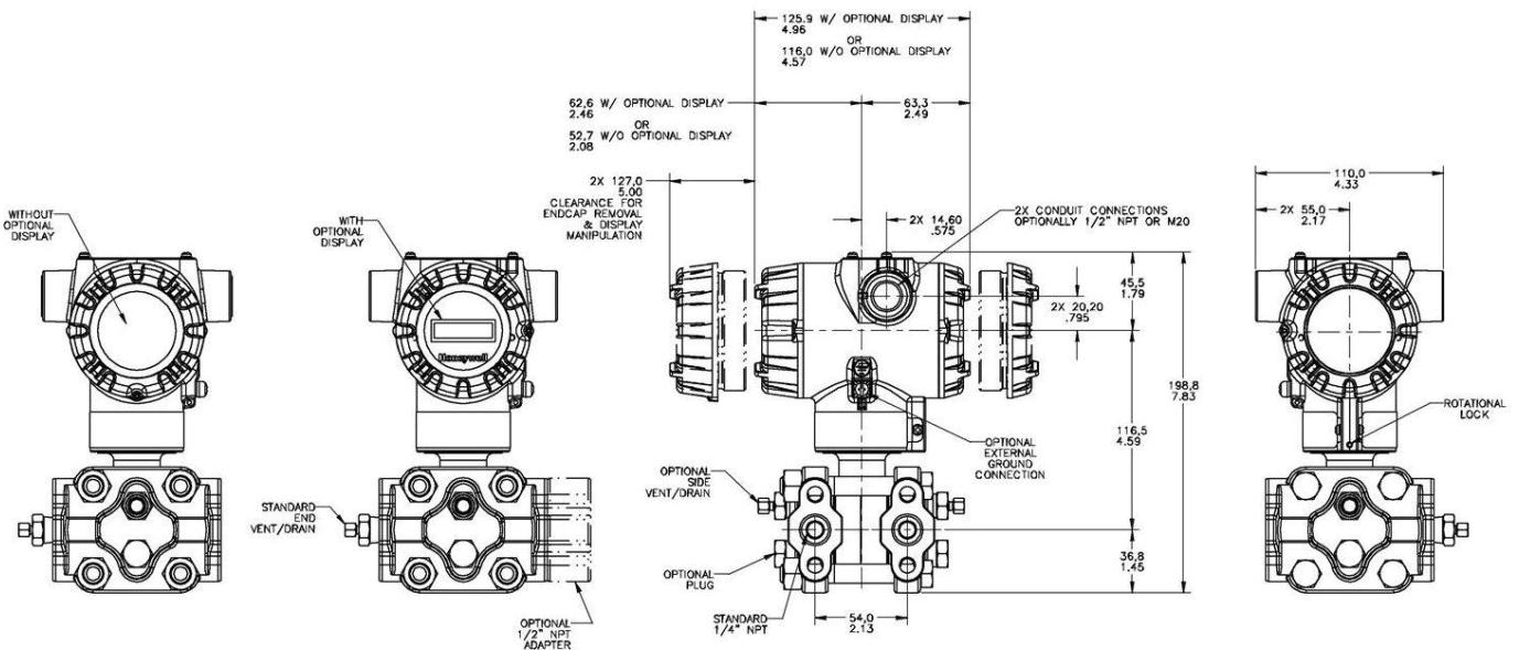
Figure 5 – Typical mounting dimensions for reference
