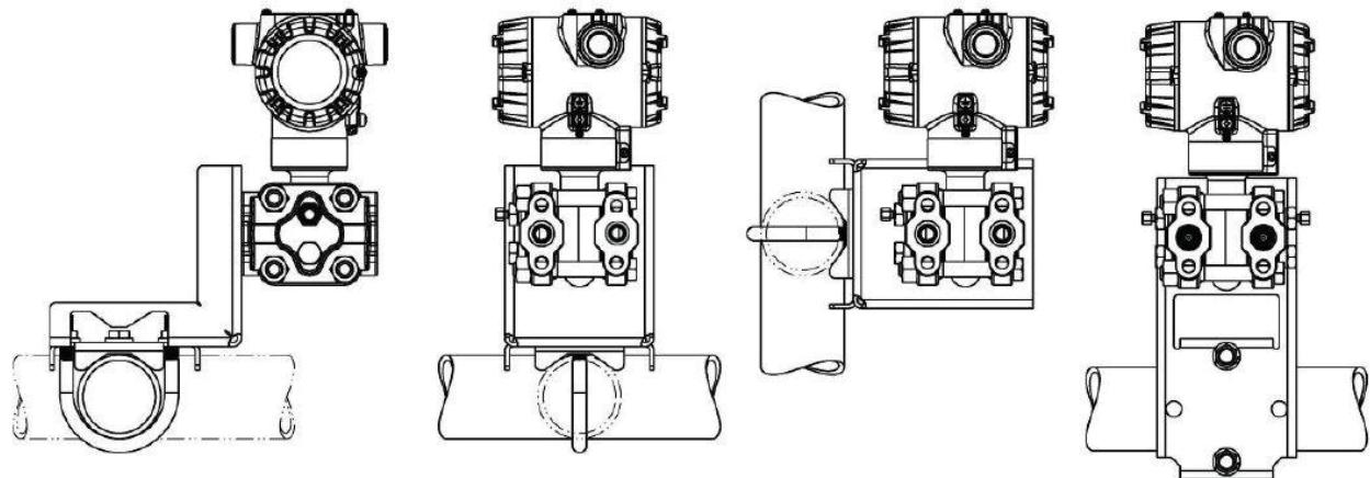
Figure 4 – Mounting Configurations
